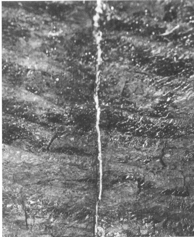
Photo 1 A hydraulic fracture propped with white sand in the roof coal at Dartbrook Coal Mine, NSW.
