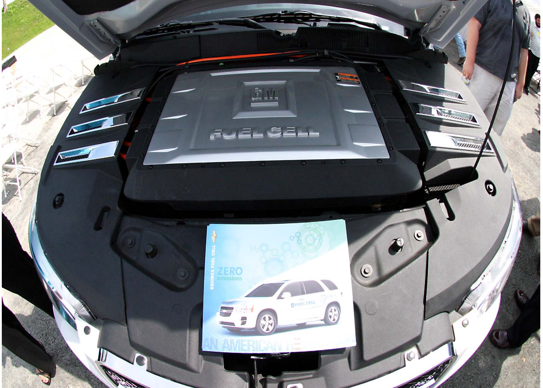
Hydrogen Fuel Cell Replaces Internal Combustion Engine
